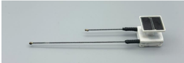
The photos to the left shows a MINI 2G P1 with elevated solar panel.
