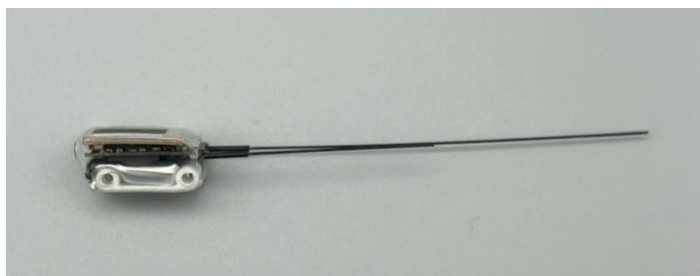
The photos to the left shows an ULRTA XC device equipped with a 3D-printed harnessing structure which weighs approx. 0.1g, and wrapped by a hot-shrinking silicon tube which weigh approx. 0.15~0.2g. This silicon tube layer can be removed using a small knife, just be careful to cut from the empty space to avoid damaging the X-coating layer.
